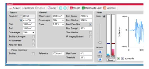
**3 AFM-IR Image Acquisition**: IR imaging maps the relative IR response across the local area of a sample, which is being irradiated at a particular wave number. The contact resonant frequency of the cantilever can be acquired simultaneously when using IR imaging mode.
