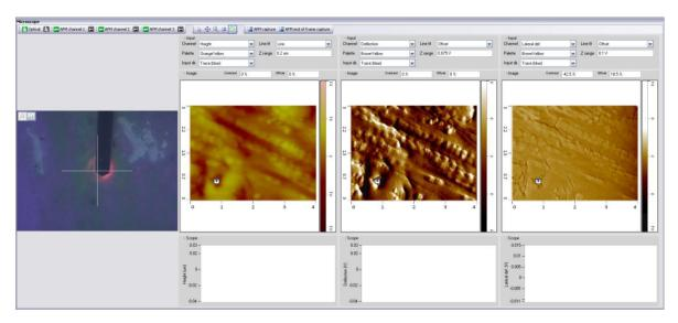
Centering the image at a specific location can be done by putting the cursor in Target mode (select the target button on the upper toolbar), then clicking on the AFM image at the desired location. This will stop the scanning and move the probe to this location on the sample. To begin scanning centered about this location, click the Target Scan button in the toolbar of the AFM Scan panel.
