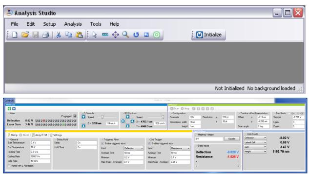
**II-3** Initialize the system by selecting the Initialize icon on the top toolbar of the software. This operation verifies communication between all the components and readies the hardware and software for use. The bottom status bar will change from "Not Initialized" to "Idle" when initialization is complete.
