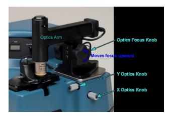
Start by adjusting the optics so that the cantilever is centered and focused in the optical view. To open the optical view in the software, select the left optics icon on the top toolbar of the Microscope Window. This view can be made full screen by selecting the right optics icon.
