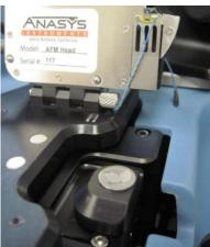
There needs to be enough clearance between the probe and sample so that they do not touch when the head is lowered back down. The safest route is to raise the head to the top of its range before lowering the head. Go to the Setup menu and select Initialize Stage.
