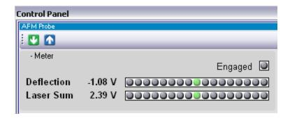
Once the green light in the light bar is illuminated, the user should **confirm that the Laser Sum value is greater than 1 V.** The exact value will depend on the type of cantilever loaded and the position of the laser spot on the cantilever.
