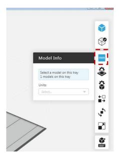
5. Then, change the material for each model by selecting the model and then selecting the 3<sup>rd</sup> box on the right-side toolbar. Just like in "Objet Studio" you can select Matte or Gloss Finish. Then you can select either "RGD", "TangoBlack", or "Vero Clear by selecting one of the 3 boxes under "Tray Materials". Do NOT worry about anything below the "Tray Material" option (outside dashed box) if you only want one material.
